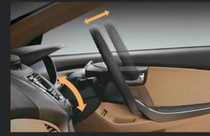
Tilt and Telescopic Steering This function allows you to adjust the steering in four different directions, thus helping you find the perfect driving position.
