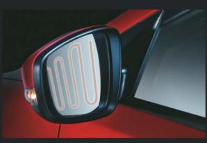
Electrically Heated Outside Mirror The outside rearview mirrors are heated electrically to help maintain visibility in extreme weather conditions.
